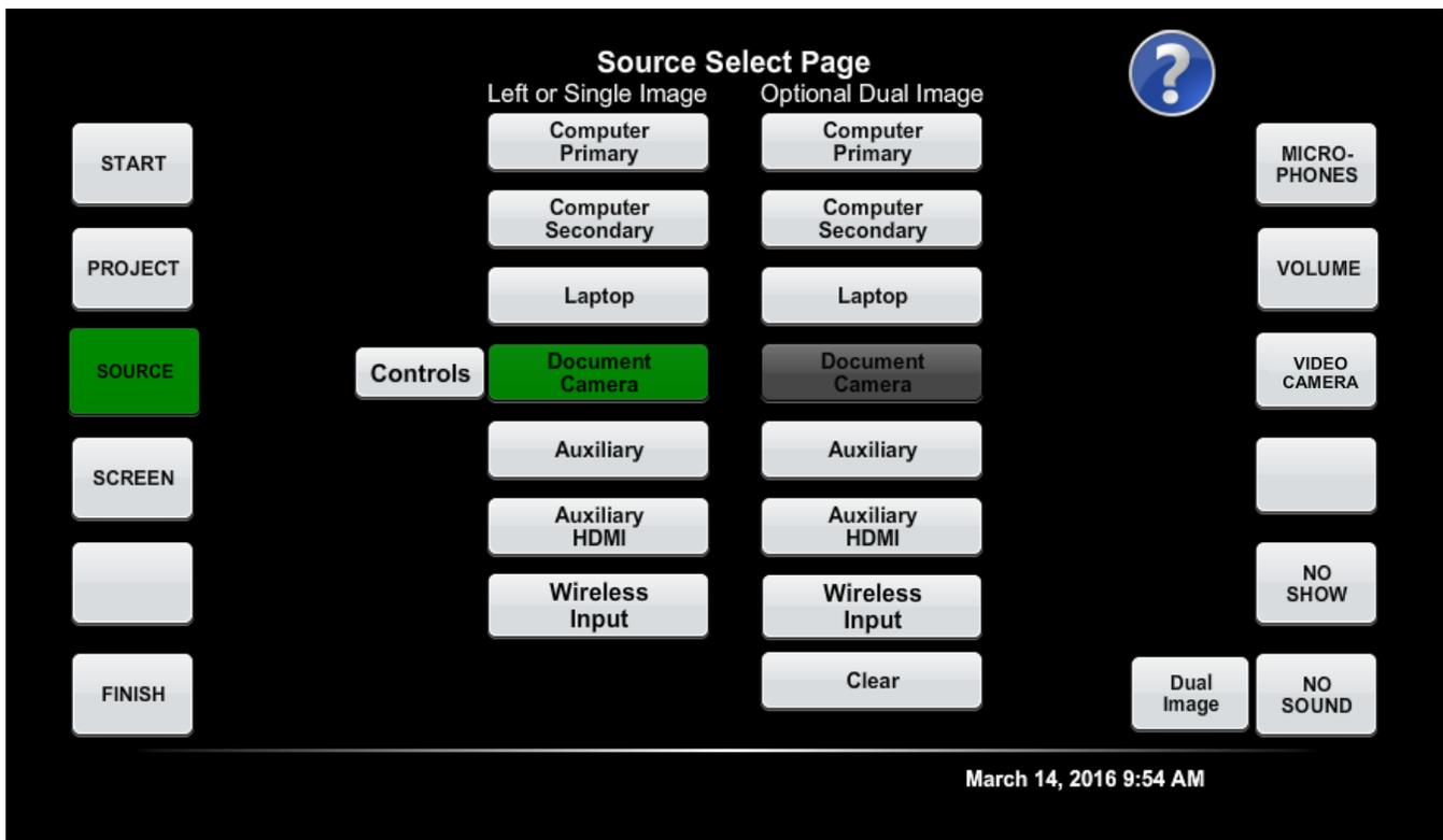
8. Source Select page for rooms with two displays. If a room has two “main” displays, the display to the audience’s left (stage right) is “Display 1” and the display to the audience’s right (stage left) is “Display 2”
