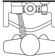
3. When the user steps away from the Object Lock Infrared Sensor, the circuit initiates the flushing cycle to flush the fixture. The Circuit then automatically resets and is ready for the next user.
