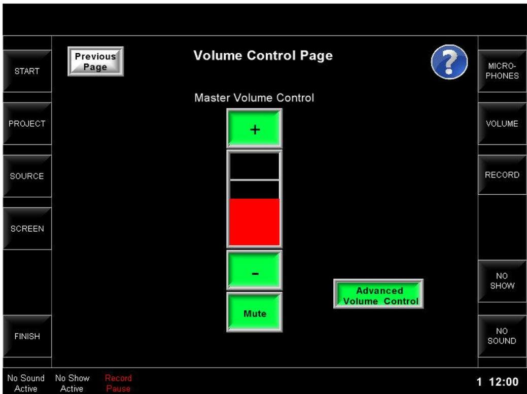
10. Advanced Volume (when raising the volume the color must go from green to yellow to red). Pressing the volume up or down buttons must also unmute the system.
