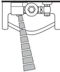
2. As the user enters the beam's effective range, 8" to 54" (203 mm - 1372 mm), the Object Lock Infrared Sensor senses the user.
