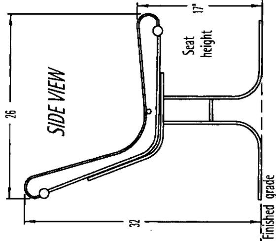
It is not recommended to locate anchor bolts until bench is in place.
