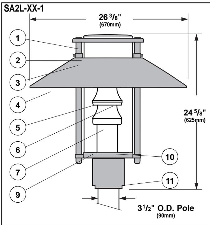
**1. Fixture Cover** - Aluminum cover with white painted interior for maximum fixture efficiency, has industrial felt gasketing for air circulation. Cover removes for lamp access.
